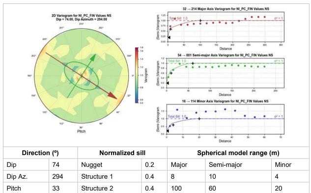
Figure 14-9: Nickel Variogram Map and Model Results for the MIN Domain
