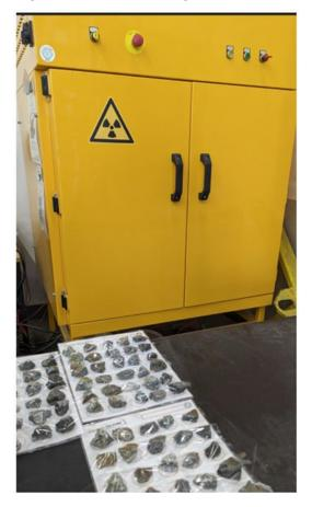
The laboratory scale sensor showed that the average densities of all lithologies were distinct, except for some particles in the low grade disseminated material and the footwall waste which had similar densities.
