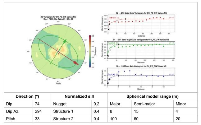
Figure 14-8: Copper Variogram Map and Model Results for the MIN Domain
