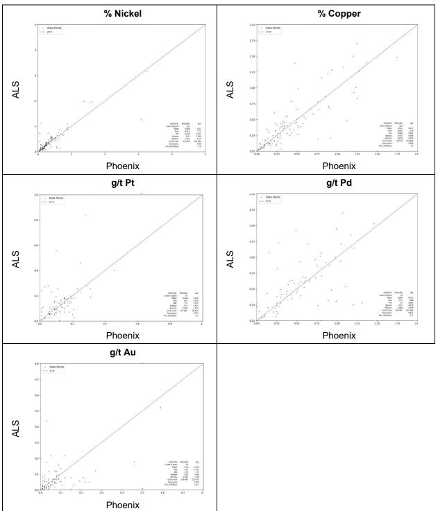
Figure 11-6: Check Assay Scatter Plots for Ni, Cu, Pt, Pd, and Au: Phoenix Mine Laboratory vs. ALS
