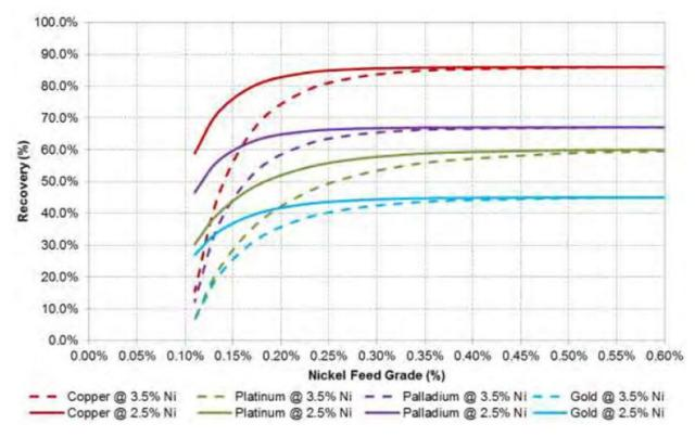
Figure 13-9: Metal Recovery Over Nickel Feed Grade Range
