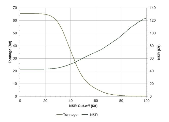
Figure 14-21: NSR Value – Tonnage Curve within the MIN domain
