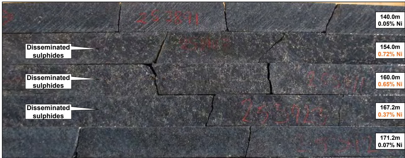
Figure 21: Norite-Hosted Disseminated Nickel-Sulphide Mineralization at Fossilik (P-058); Borehole MQ-15-077
