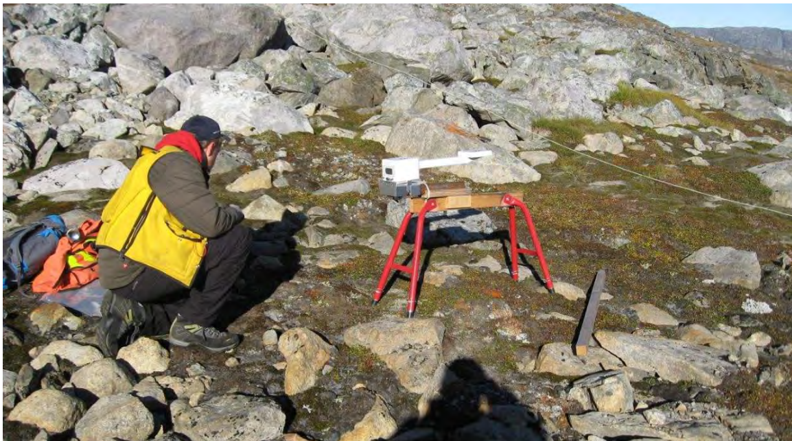
Figure 63: Field Mounted APS Unit (white) Used to Position Foresites
