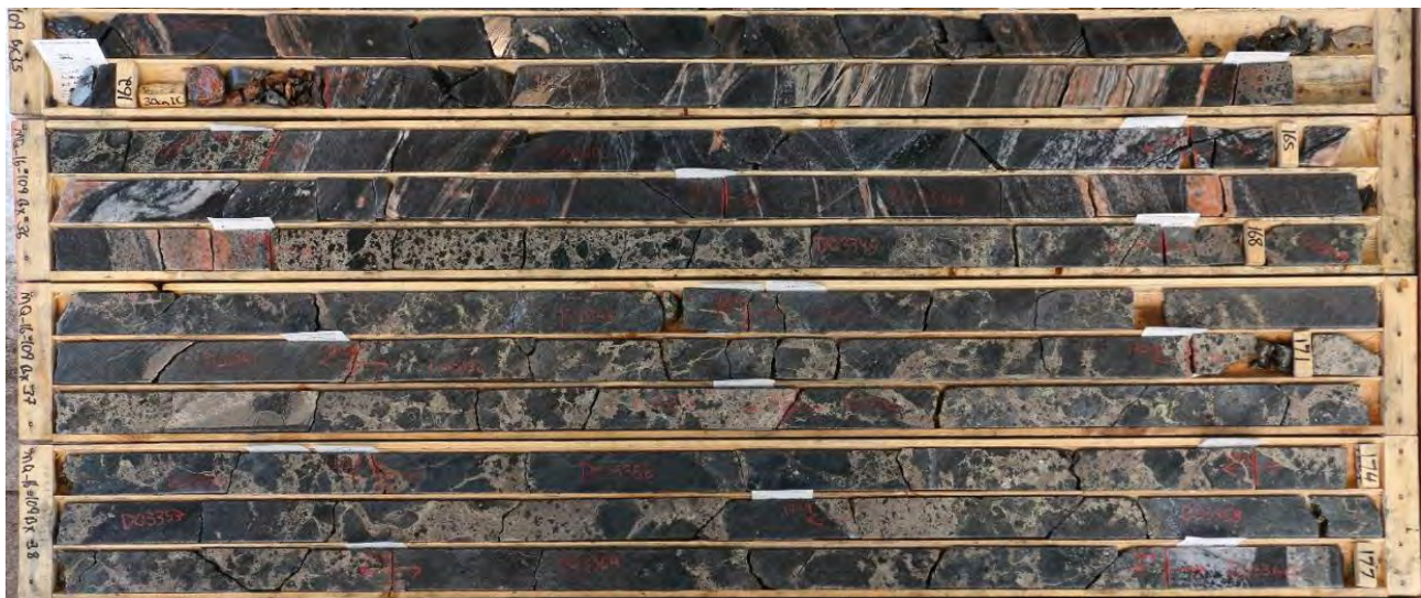
Figure 33: Remobilized Sulphide Zone at P-013 SE; Borehole MQ-16-109
