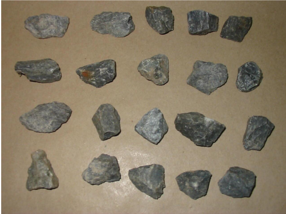
Figure 4 – A Typical Set of Particles for Breakage (Particle Selection Method)
