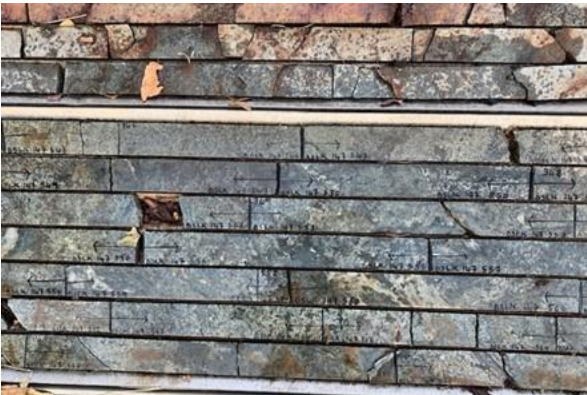
Figure 12-5: Typical Taxitic Gabbro (Drillhole DSLK147)
