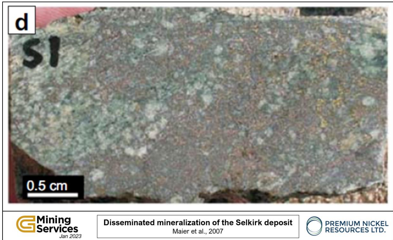
Figure 7-6: Disseminated Chalcopyrite–Pyrrhotite Mineralization Collected 4 m Below Massive Sulphide Body. Sample S1, Selkirk
